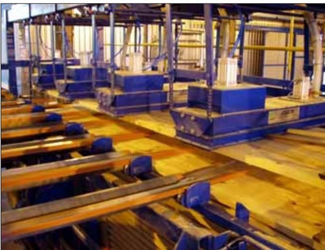
3. Destacking layer transversally using vacuum
