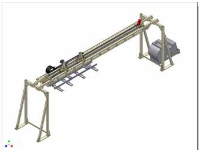
4. Destacking layer longitudinally using vacuum
