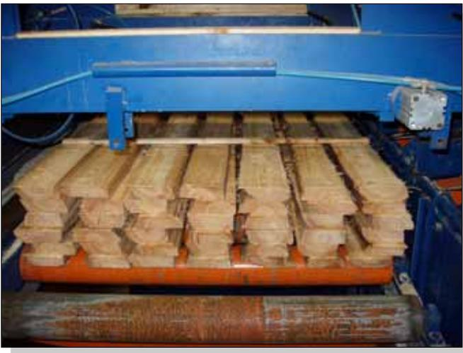
11. Stacking of layers of planks resawn in to slats
