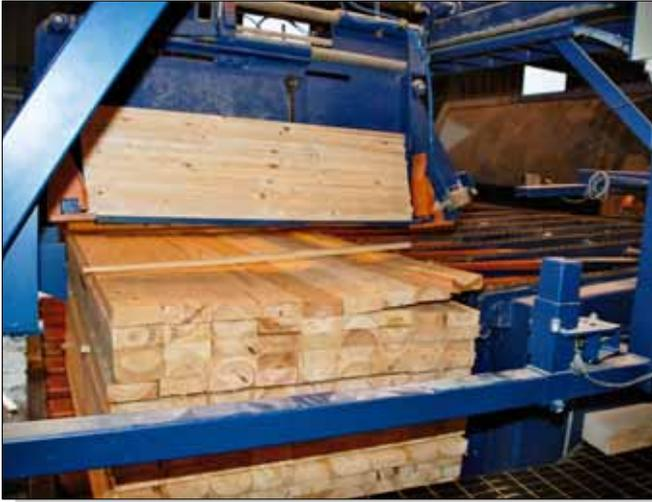
5. Standard stacking machine with stick laying
