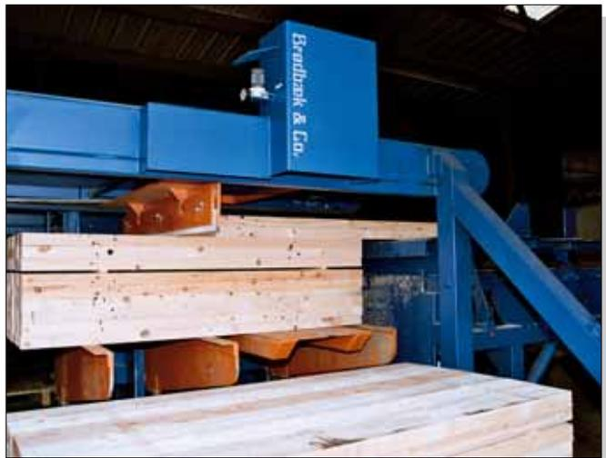
2. Destacking layer longitudinally using push bar
