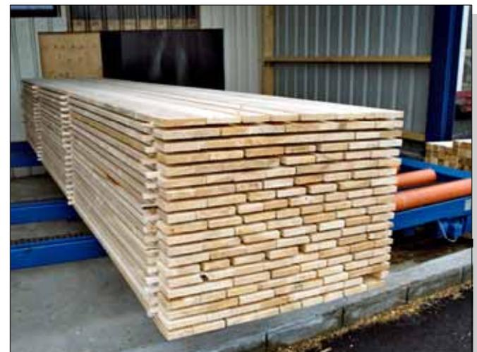
9. Stacking of mixed widths using horizontal spacing – ideal for kiln drying
